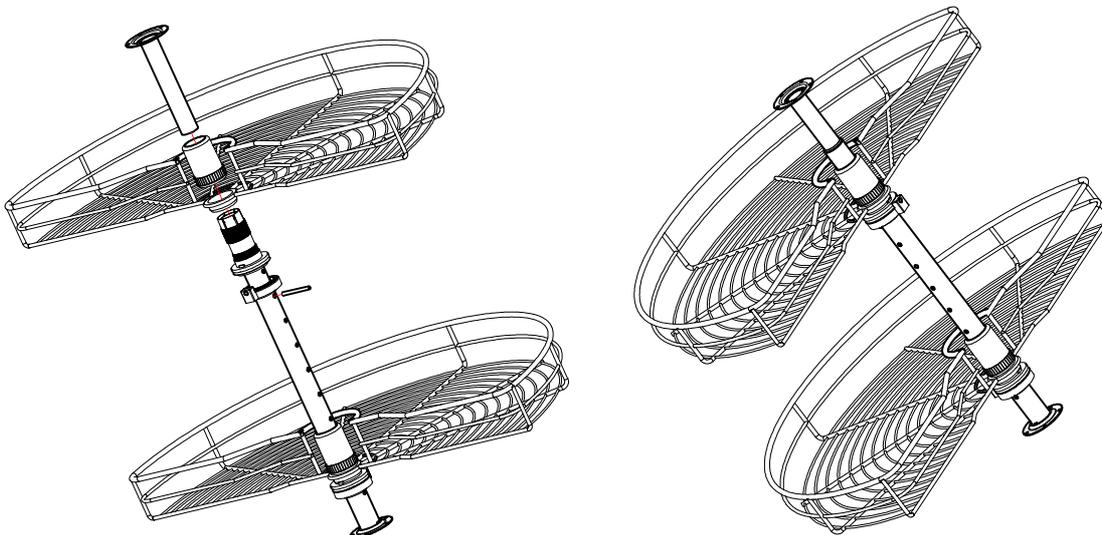
3. Slide the short tube into the long tube and attach to the top of the cabinet.
