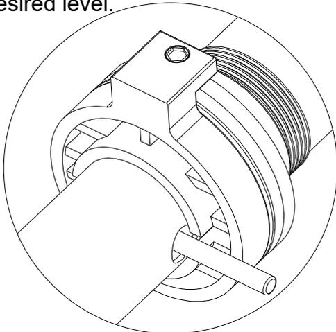
To adjust the rotation strength, tighten hex bolt with Allen key.
