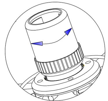
Screw on with moderate intensity / don't screw on tight.
