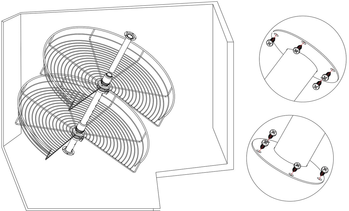
To adjust the position of basket, insert pin at desired level.
