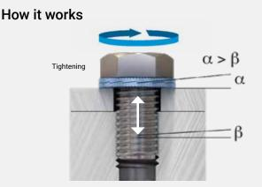
When the fastener is tightened, the cams lock and the serrations on the outer faces of the washers grip into both the fastener and the clamped part, creating clear impression marks in both. Clamping load has been created by the bolt, keeping the assembly locked in place.
