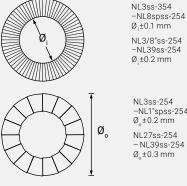
NL3ss-254 –NL1"spss-254 Ø<sub>o</sub>±0.2 mm NL27ss-254 - NL39ss-254 Ø<sub>o</sub>±0.3 mm
